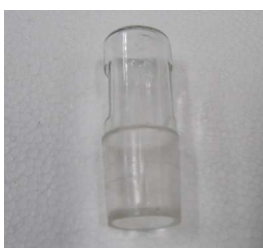
Blind stopper 29/32 for addition funnel
