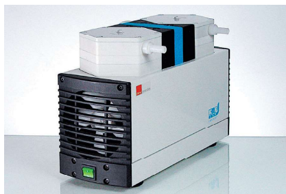
Vacuum mebrane pump N-820 Special for solvents Flow volume 20 litres/minute. Vacuum limit 8 mbar. PTFE rotors. PTFE coated membranes, valves in FFPM, motor protection level IP-44 Part number 5910009
