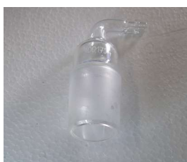
Stopper 29/32 with outlet 10mm at 90°C
