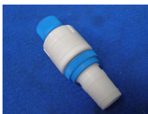
Guide for PTFE stirrers 29/32 Ø 10 MM High chemical resistance Low vacuum (5mmHg) Pressure (3-5 psi) High performance PTFE/PEEK/glass precision bearing seal Internal anti-whip sleeve Part number 1001788
