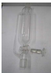
Addition funnel 250ml, compensated pressure DIN29 / 32
