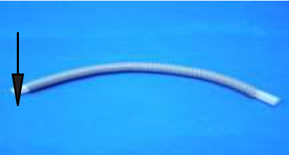
Silicone pipe External diameter 14 mm. Internal diameter 8 mm Part number 46041
