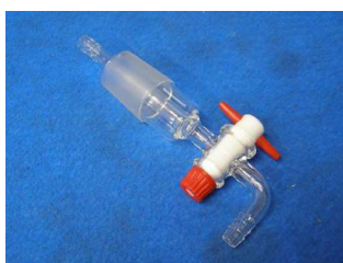
Load faucet 29/32 Step 4mm Olive 12/13 Part number 1001793
