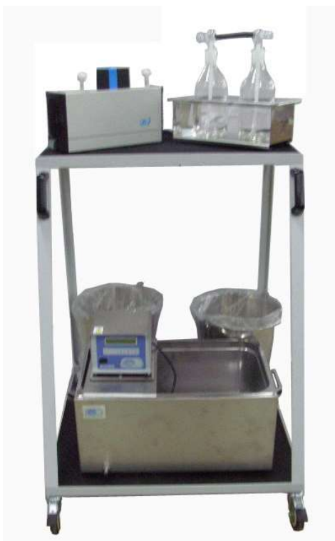
Digiterm TFT, Vacuum pump, Scrubber & steel cubes
