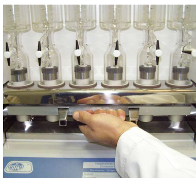
Placing thimbles on the extraction unit.
