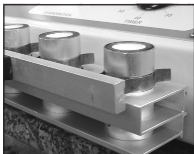
Extraction thimbles ready to insert into the extractor.
