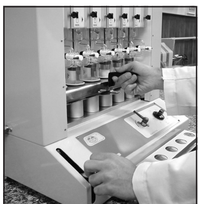
Placing the beakers on the extraction unit
