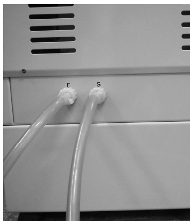
Fig 4.3: Inlet and outlet water connections
