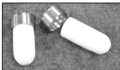
Mounting the thimble holder
