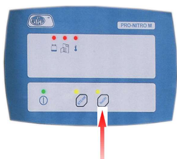
Manual NaOH adding during distillation
