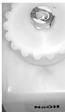
Clean periodically the NaOH tank and fixative solution tank hose connector.
