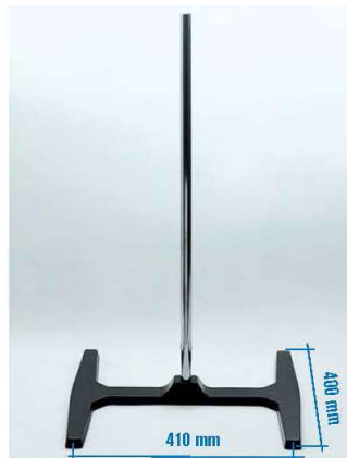
DOUBLE BASE SUPPORT T "MAXI" Rod of AISI 304 stainless steel of 20 Ø x 800 mm high. Designed to support weights up to 20 Kg at 300 mm height from the base. Useful for stirrers. Weight: 7 Kg. Part No. 6000410
