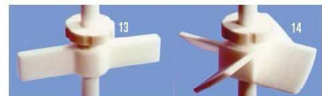
ADJUSTABLE HEIGHT SHAFT STIRRERS Shafts made of AISI 304 stainless steel coated in PTFE and PTFE stirrer paddles. Shaft: 8 mm Ø. Adjustable height paddles using a locking thread. Can be used with differing paddles on the same shaft to create a multiple mixing action.
