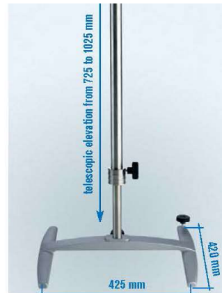
DOUBLE BASE SUPPORT T TELESCOPE Stainless steel base AISI 304 of 32 mm Ø. Telescopic elevation from 725 to 1025 mm. Maximum support weight 20 Kg. Actual weight: 7.7 Kg. Compatible with Part No. 5057022 (See page 166). Part No. 5057011
