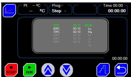
Run screen operating with temperature profile.
