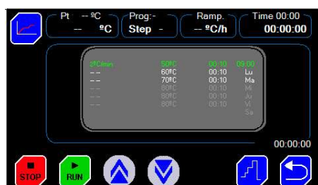
Fig 7.3. Run screen operating with temperature profile.
