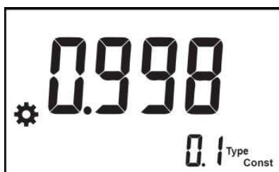
Fig. 5-10 Constant Type is 0.1, Cell constant is 0.998
