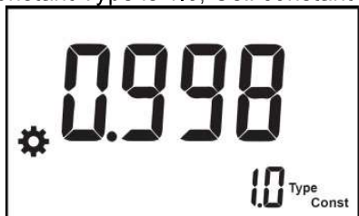
Fig. 5-9 Constant Type is 1.0, Cell constant is 0.998
