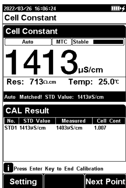
Figure 5-4 Electrode cell constant calibration information
