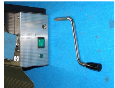
Insert the sealing lever on his squared shape fixing hole.
