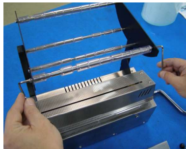
Fix the two bigger rods on the black stands upper holes with the M5 screws.
