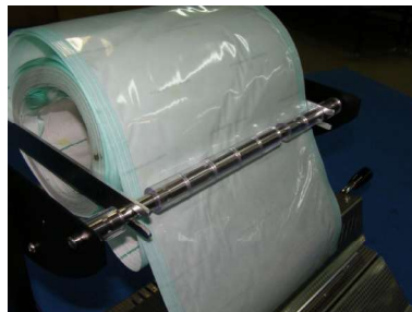
Inserting the paper to the sealing head.
