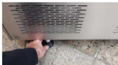
Locking Wheels of 150L autoclave
